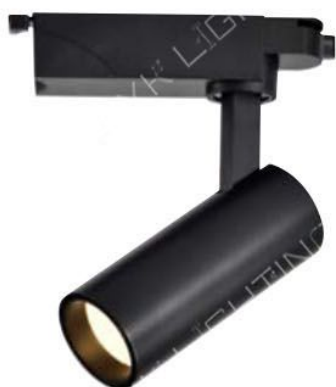
G-129-1 4000 Ø50 H120mm COB LED 10W 3000K 4000K 6000K
