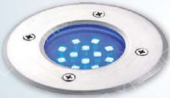
LV-11-5234 2800 W104mm H40mm 附LED 12顆 3WX1、藍光、全電壓 304不鏽鋼面板、預埋盒自購 嵌入孔：Ø94mm H45mm
